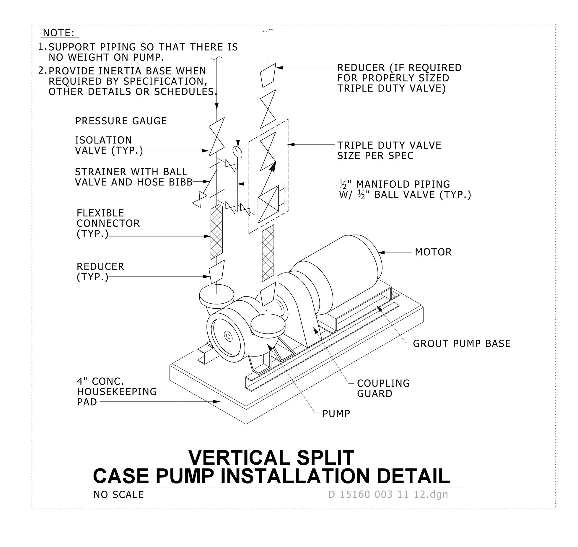
DESIGNER NOTE: FOR VARIABLE VOLUMNE SYSTEMS, DELETE TRIPLE DUTY VALVE AND SHOW A CHECK VALVE INSTEAD.
